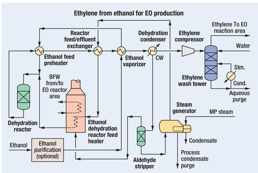
FIG. 8 Flow diagram of EO/EG plant using ethanol as the feedstock.
