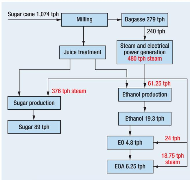
**FIG. 9** An integrated biorefinery uses sugar cane to process EO and other downstream derivatives.
