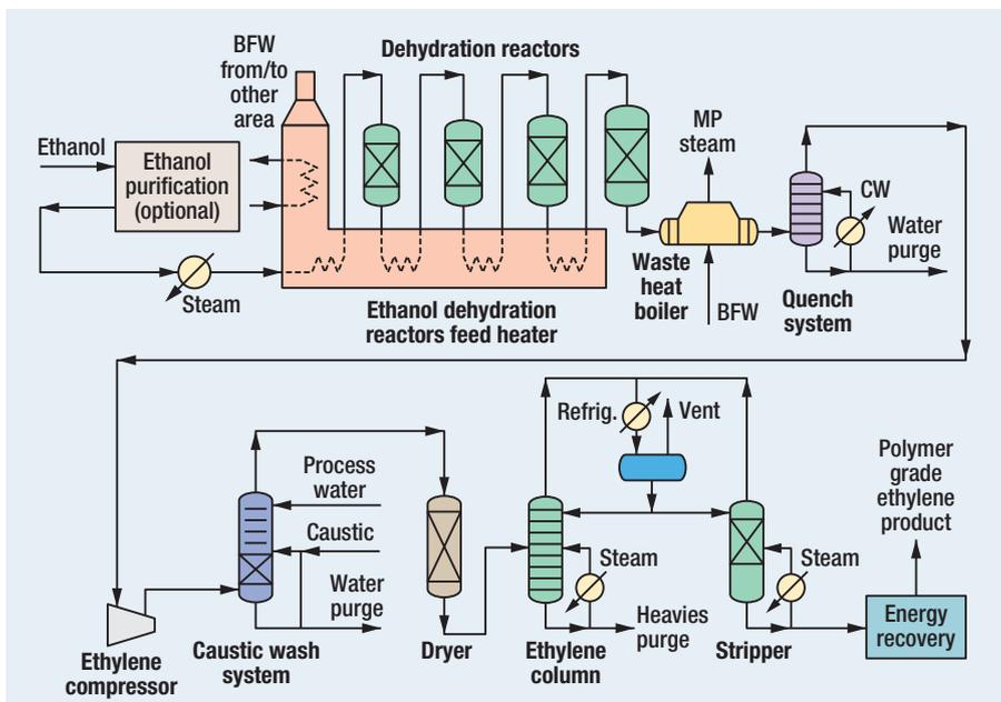
FIG. 7 Flow diagram of polyethylene based ethanol as the feedstock.
