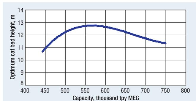
FIG. 7 Optimum catalyst-bed height vs. single reactor capacity.
