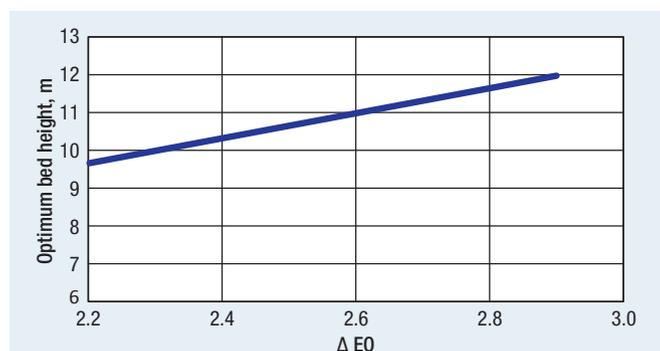
FIG. 6 Optimum catalyst bed height vs.  $\Delta\text{EO}$ .
