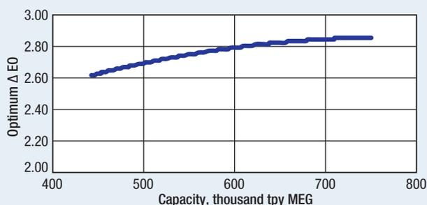
**FIG. 9** Optimum  $\Delta$ EO vs. reactor capacity.
