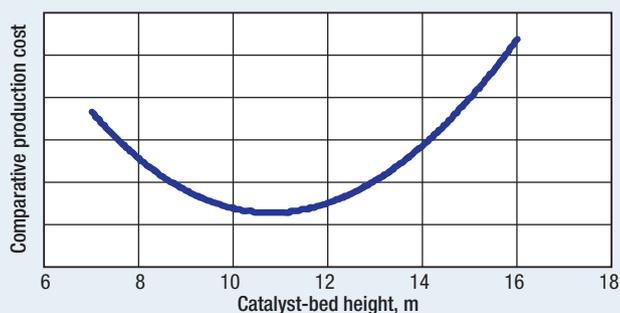
**FIG. 3** Production costs vs. bed height for EO reactor.
