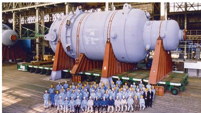
**FIG. 2** Photo of a typical large modern EO reactor.
