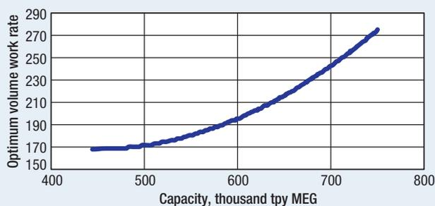
**FIG. 8** Optimum work rate vs. single reactor capacity.
