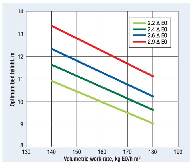
FIG. 4 Optimum catalyst bed height based volumetric work rate.
